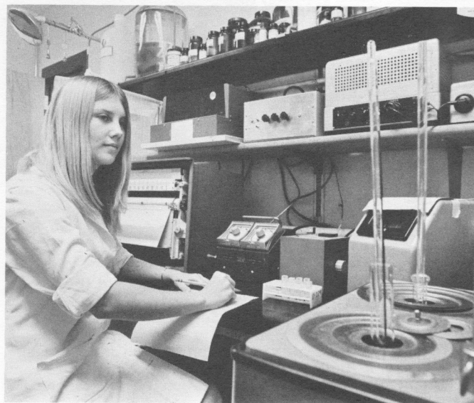
DOROTHY DAY of Tempe works with a spectrophotometer to measure difference in light intensity of the starting material and the final product during an enzyme catalyzed reaction. With this equipment it is possible to measure the amount of enzyme in a solution or tissue extract.
