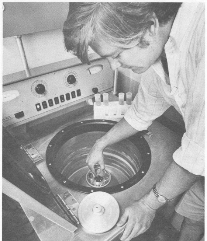
ROBERT INGALLS of Tempe places an enzyme solution in a centrifuge. The machine will spin the solid materials to the bottom of the container, leaving a purer enzyme in the solution. If it were mud he placed in the machine, the tube would come out with dirt on the bottom and clear water on top.
